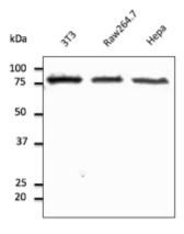
Anti-Calnexin - ER membrane marker Ab at 1/2,500 dilution; lysates at 50  $\mu g$  per lane; Rabbit polyclonal to goat IgG (HRP) at 1/10,000 dilution;
