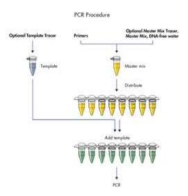
Figure 1. UCP Multiplex PCR procedure using tracer dyes.
