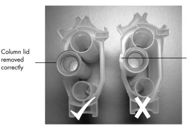
Column lid removed incorrectly; part of lid still attached
