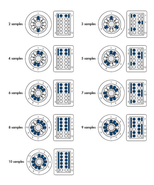
Figure 9. Loading the centrifuge and shaker. Centrifuge and shaker positions are shown for processing from two (2 samples) to ten (10 samples) samples. One or 11 samples cannot be processed.
