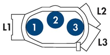
Figure 7. Positions in the rotor adapter. The rotor adapter has three tube positions (1-3) and three lid positions (L1-L3).
