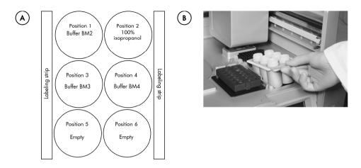
Figure 4. Loading the reagent bottle rack. [A] Schematic of positions and contents of bottles in the reagent bottle rack. [B] Loading the rack onto the QIAcube Connect.
