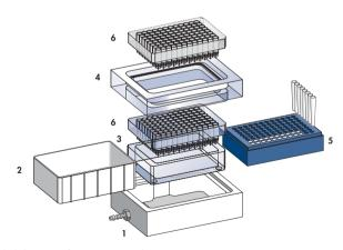
Figure 3 Exploded diagram of QIAvac 96 and components
