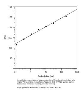
**Figure 1.** Acetylcholine dose response was measured in a 96-well solid black plate with Amplite<sup>™</sup> Fluorimetric Acetylcholine Assay Kit (Cat. # 11403) using a Gemini fluorescence microplate reader (Molecular devices).
