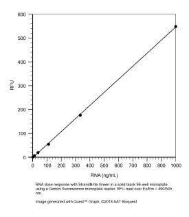
**Figure 1.** RNA dose response with StrandBrite Green in a solid black 96-well microplate using a Gemini fluorescence microplate reader. RFU read over Ex/Em = 490/545 nm.
