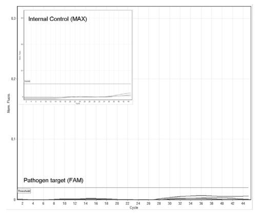
Figure 6. Amplification curves on the Rotor-Gene Q do not exceed the threshold for either of the pathogen target and the Internal Control (inset), indicating that amplification has failed.
