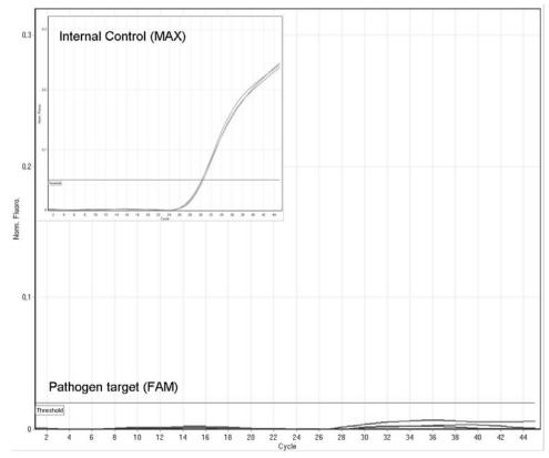
Figure 5. Typical amplification plots on the Rotor-Gene Q showing no signal for three replicates of a pathogen target with successful amplification of the Internal Control (inset) at the same time, indicating absence of the pathogen target in the sample.
