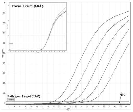
Figure 4. Typical amplification plots on the Rotor-Gene Q for different concentrations of a pathogen target and for the Internal Control (inset).
